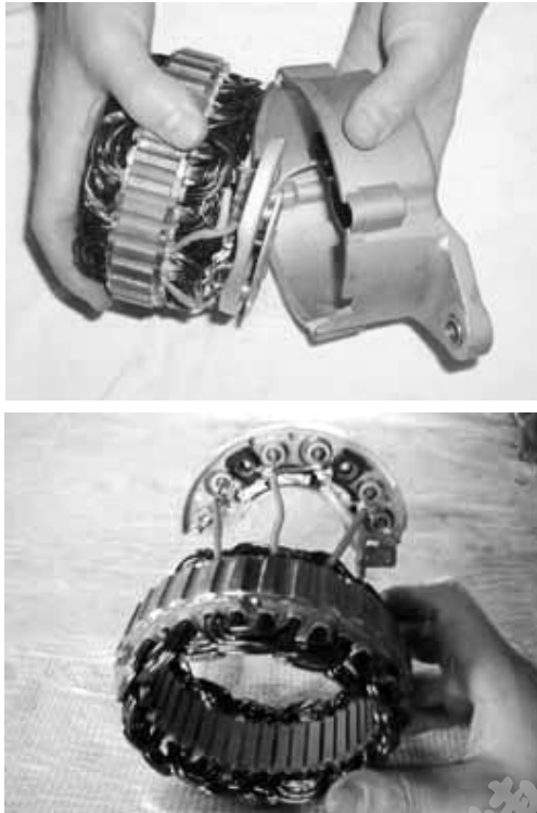
圖8 鬆開A線頭、用電烙鐵將焊錫熔解
